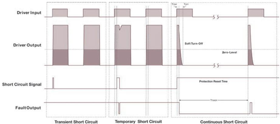
In block two, a temporary short circuit condition extends past the  $T_{TRIP}$  limit ( $>2.6 \mu s$ ) and triggers a shutdown. When an actual short circuit is detected (at the end of  $T_{TRIP}$ ), the driver provides a soft shut down. This will limit the transient voltage surge that occurs when large short circuit currents are interrupted. The default soft shutdown time is 5.0  $\mu s$ , which should work for most applications.
