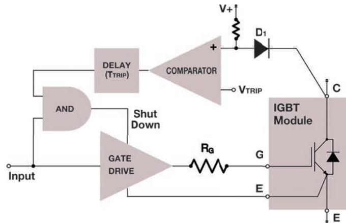
The IGD962-5A provides short circuit protection by means of an on-state collector-emitter voltage sensing circuit. This type of protection is often called "Desaturation Detection". A block diagram of a typical desaturation detector is illustrated at left.
